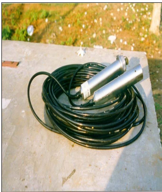
Figure 6.4: Photograph of components of DWLR showing the pressure sensor, cable and connector
